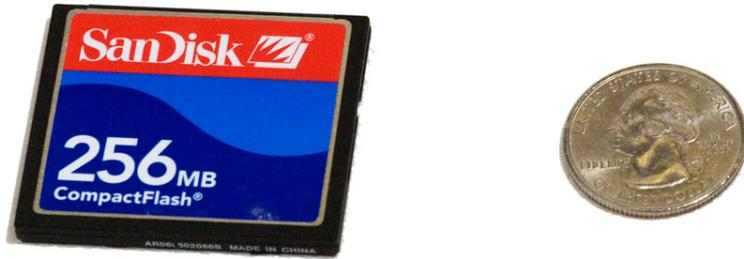
Figure 5.5: A Compact Flash card used by the Voter iVotronic and AutoMARK
