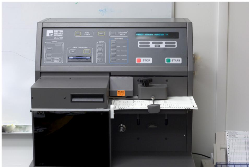
Figure 5.8: The ES&S M650 centralized optical scan ballot counter
